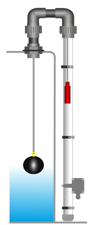
Silotank's Cat and Mouse Tank Level Indicator allows an easy and precise reading of the tank level. The float within the tank is suspended by a cable, supported by 2 No 90° PVC elbow pulleys in a special 'no jump' system. The counter pulley system, the volume of liquid in the tank is shown within a clear PVC pipe which is installed externally, parallel to the tank.
